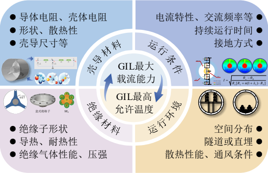
图 A2 GIL 载流量关键影响因素 Fig. A2 Key factors of GIL current carrying capacity
